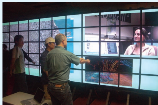
LambdaVision 100-Megapixel display and SAGE (Scalable Adaptive Graphics Environment) software developed by the Electronic Visualization Laboratory at the University of Illinois at Chicago. Major funding provided by NSF.
